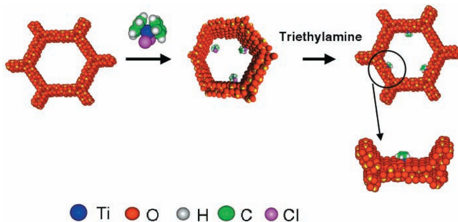
FIGURE 2. Color graphic illustration of the various initial steps in the preparation of the Ti IV -centered active site. The titanocene dichloride in the presence of the triethylamine becomes anchored via the silanol groups on the inner wall of the mesoporous silica (MCM-41) to form a half-sandwich compound. This, on calcination, forms the tripodally anchored Ti IV active center, designated Ti IV MCM-41. 24
